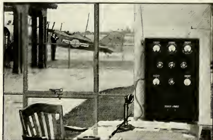
10A radio telephone transmitter and microphone in manager's office at Burbank. Dispatcher (seen at end of canopy) is giving instructions to pilots through a second microphone.
